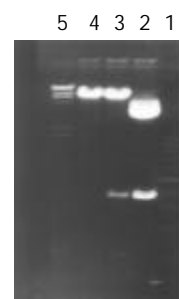
Figure 1 pAd-p27kip1 appraisal 1 200 bp ladder Marker: 200, 400, 600, 800, 1 000, 1 200, 1 400, 1 600, 1 800, 2 000 bp. 2, pCMV5p27kip1 (kpnI+BamHI): 690 bp segment. 3, pAd-p27kip1(kpnI+BamHI): 690 bp and 8 800 bp segment. 4, pACCMVPLPA (kpnI+BamHI): 8 800 bp segment. 5, Hind III marker: 2 027, 2 322, 4 361, 6 557, 9 416, 23 130 bp.
