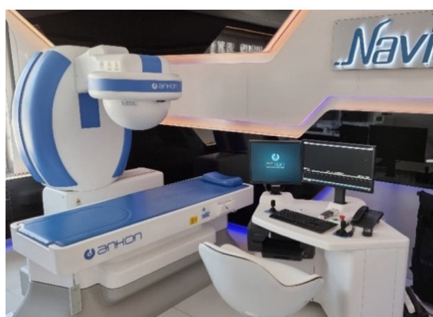
Figure 1 Robotic C-arm, investigation table, and computer workstation for magnetically controlled capsule endoscopy.
