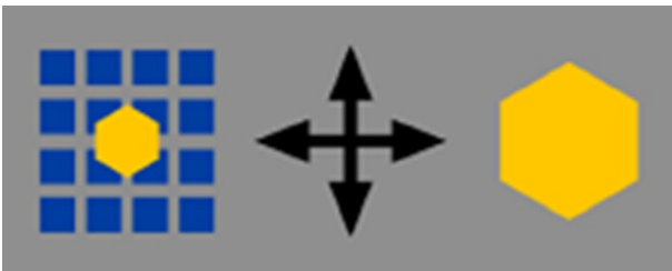
Figure 2 Electronic magnification simply moves the image closer on the display and results in a decreased number of pixels composing the area of display, with no improvement in resolution.
