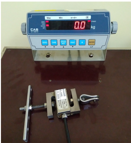
Figure 4 Device for recording breakout force with a strain gauge.
