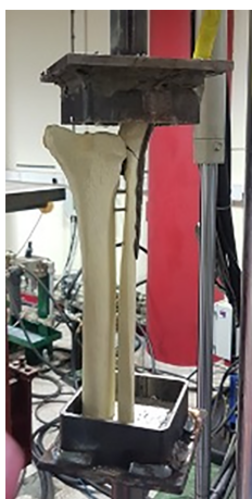
Figure 3 Fibula pro-tibia construct of ankle fracture sawbone model mounted on the electromagnetic test frame (MTS 858 Mini-Bionix test machine, MTS Corp, Eden Praire, MN, United States).
