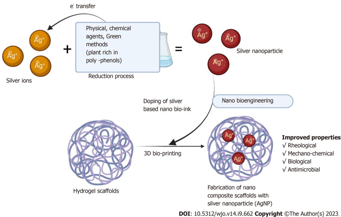
Figure 2 Doping of silver nanoparticles in scaffolds.
