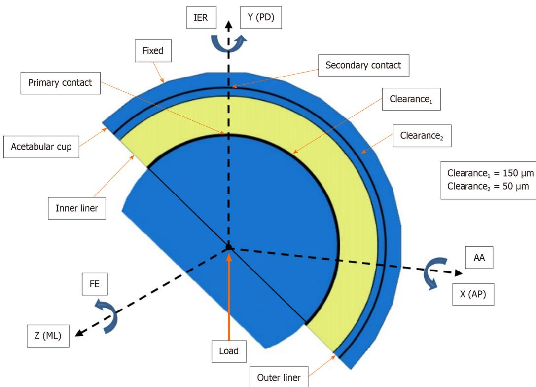
Figure 4 The DM hip joint reference frame. AP: Anterior-Posterior; IER: Internal-External Rotation; PD: Proximal-Distal; FE: Flexion-Extension; ML: Medial-Lateral; AA: Adduction- Abduction.
