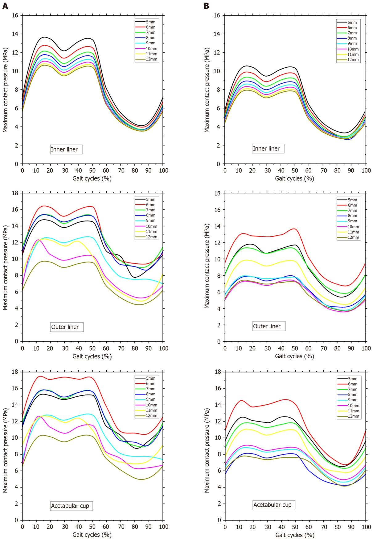
**Figure 7** Maximum contact pressures based on gait cycles. A: 28 mm head diameter; B: 36 mm head diameter.
