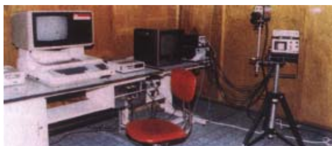
Figure 1 AGA-782 infrared thermovision system
