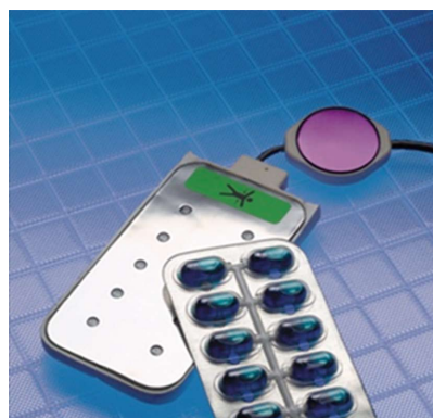
Figure 4 One defibrillator electrode with ten gel capsules inserted in, and one non-adhesive electrocardiogram electrode.
